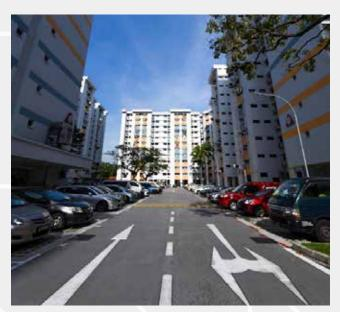
From 2019 to end-2020, two blocks in Bukit Purmei served as a testbed to determine if heat-reflective paint, applied on the building facade and carpark surface, is able to reduce ambient temperature by 2 degrees. Known as CoolPaint, it contains transparent polymeric beads that are capable of reflecting the infrared portion of solar radiation, allowing the painted surfaces to absorb less heat during the day.
