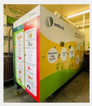
The reduction of food waste at our hawker centres has begun with the pilot installation of a food digester machine at Redhill Food Centre. The machine converts food waste into compost and non-potable water, while remaining odour-free with its air purification system. From January 2021 to July 2021, the machine has processed 11,200 kg of food waste.
